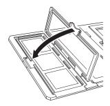
4. Place the holder on the document table, and align it with the notch on the transparency guide, as shown below.
